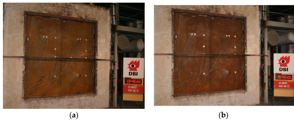
Figure 5. (a) H-120 bulkhead at the beginning of fire test. (b) H-120 bulkhead at the end of fire test.
