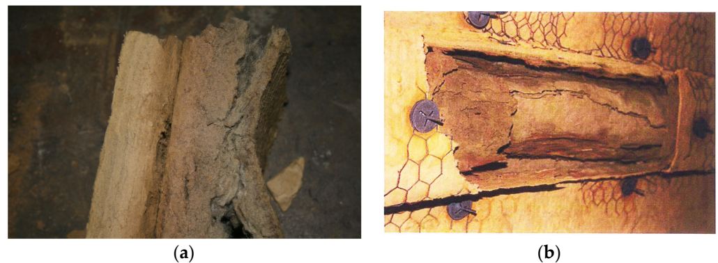
Figure 6. (a) Mineral wool after fire test of H-120 bulkhead. (b) Mineral wool after fire test of H-0 bulkhead.
